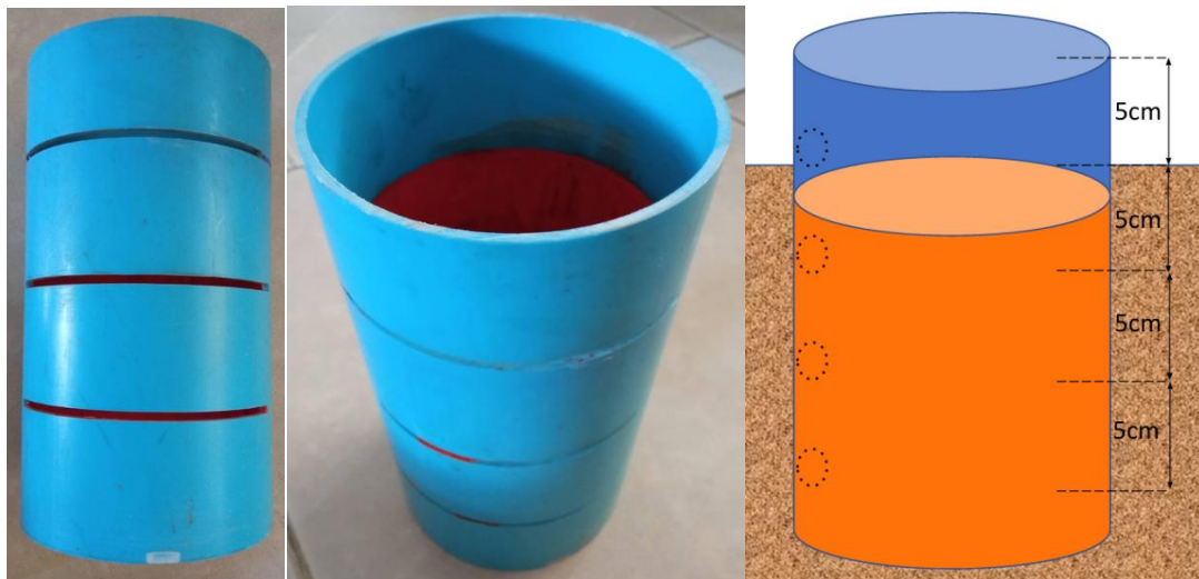
Figure 2: Perforated PVC pipe for monitor the subsurface water level
